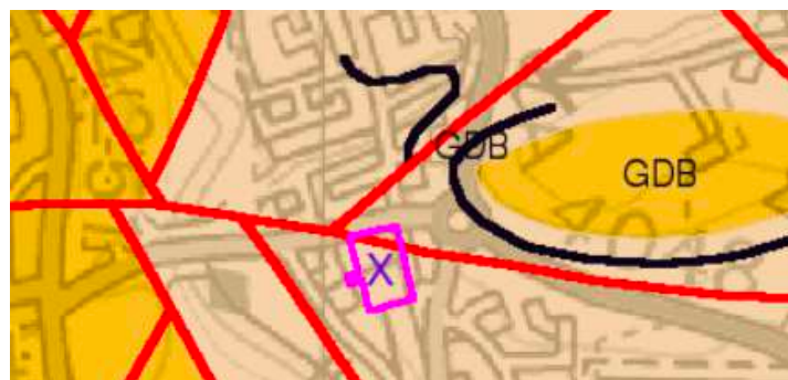
Extract from Envirocheck Report showing faulting on and around the site
